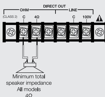
NOTE: Only connect one output – either 100V or 4Ω
